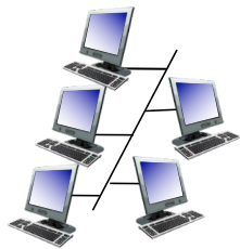
shared wire (e.g., cabled Ethernet)
